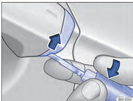
Fig. 54 Manilla de la puerta del conductor: levantar la caperuza.
